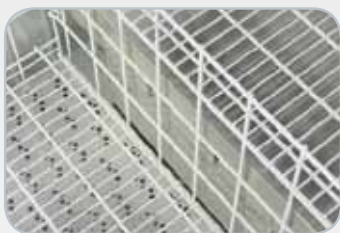
False bottom for air circulation
